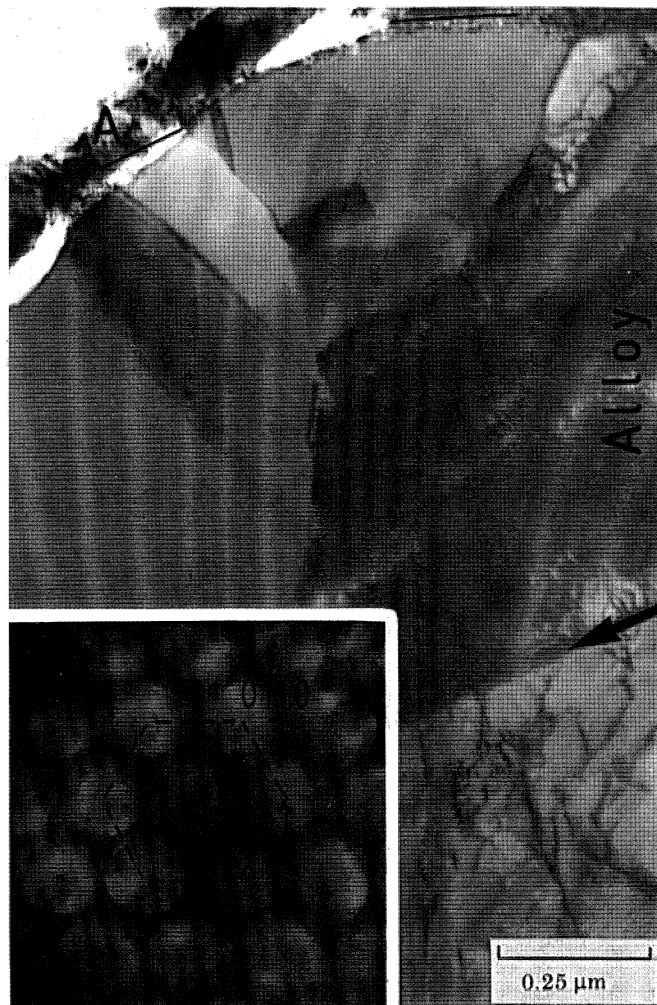
FIGURE 14. Fe-10Cr-34Ni oxidized in air for 1000 h at 600 °C showing a thin layer of 'protective' oxide sandwiched between the alloy and supportive nickel plate, as at A. Note that the alloy shows partial recrystallization to a depth approximately 1 μm beneath the scale, as arrowed.
