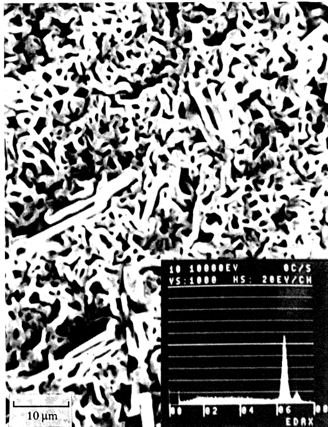
FIGURE 4. Scanning electron micrograph and 20 kV EDS analysis (Fe:6.398 keV) of the surface of the scale formed on Fe-10Cr-10Ni in 1% CO-CO 2 after 1000 h at 600 °C.
