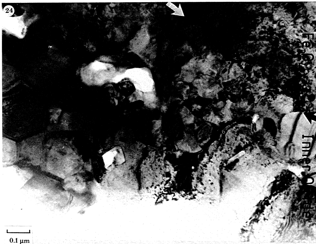
FIGURE 23. Microstructure of the magnetite formed on Fe-10Cr-20Ni after 125 h oxidation in 1% CO-CO 2 at 600 °C. The image shows the scale at the oxide-gas interface, where the magnetite-nickel plate interface is marked. (The plate is used in the preparation of the 'edge-on' foils.) Grain boundaries in the magnetite are arrowed, which are regions where enhanced oxide growth has occurred, leaving cavities in the surface of the scale, as at A.
