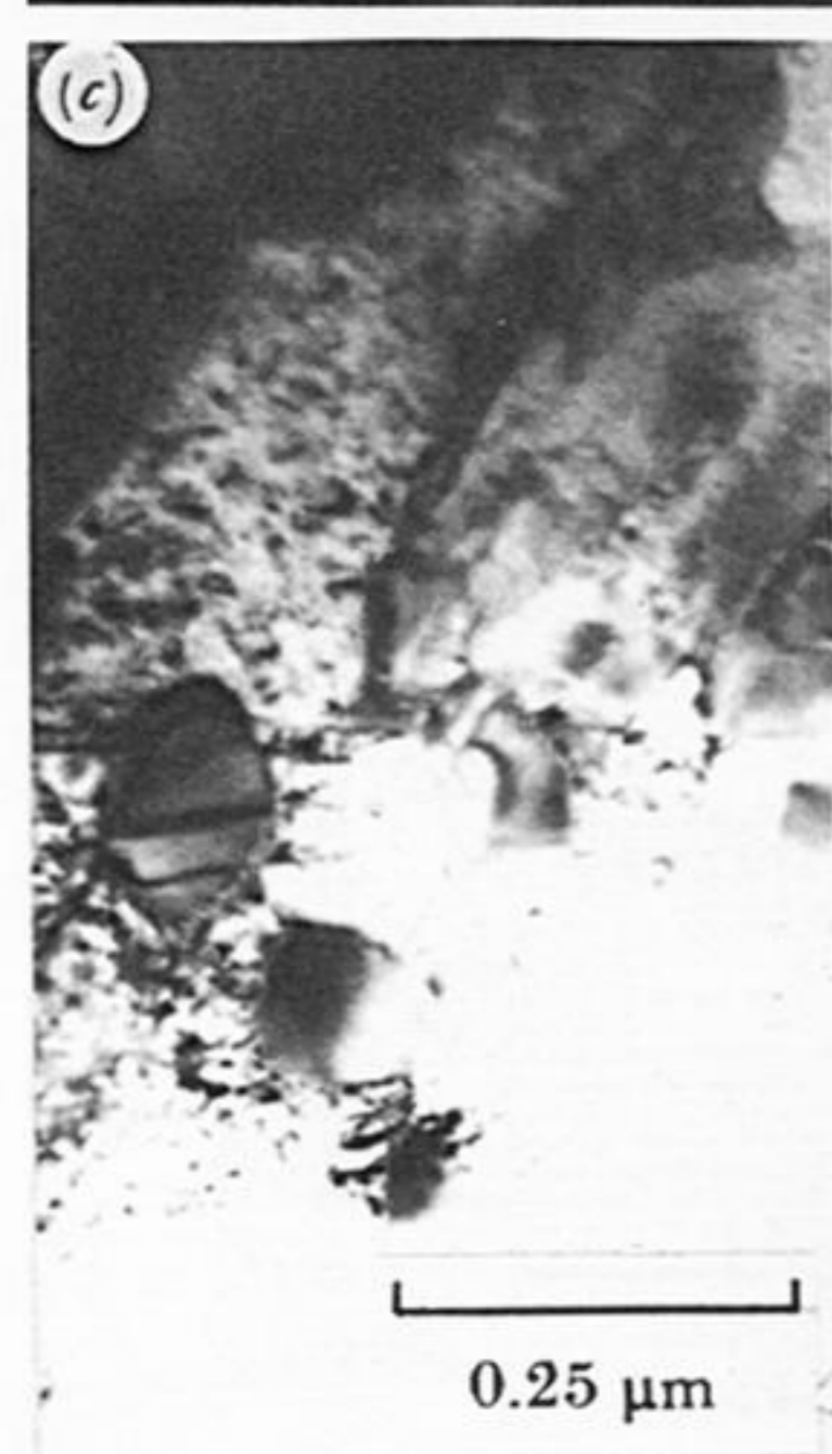
FIGURE 20. Fe-10Cr-10Ni oxidized in 1% CO-CO 2 for 125 h at 600 °C. 'Edge-on' TEM showing the microstructure of the oxide approximately 100 μm beneath the duplex oxide interface. (a) Bright-field micrograph showing ferrite, austenite and M 23 C 6 carbides, as marked; (b) (012) α //(111) γ //(111) M 23 C 6 diffraction pattern; (c) Bright-field and (d) dark-field (imaged with a (200) ferrite reflection); (e) dark-field (imaged with a (220) austenite reflection); (f) dark-field (imaged with a (220) carbide reflection).
